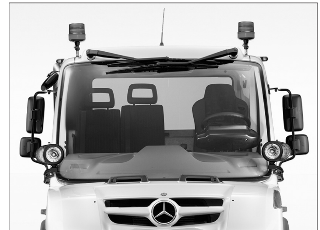
Rotating beacons and additional headlamps
