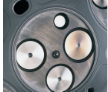
The engine breathes better with three valves per cylinder. A fourth valve is utilized for the optional MBE 900 compression brake.
