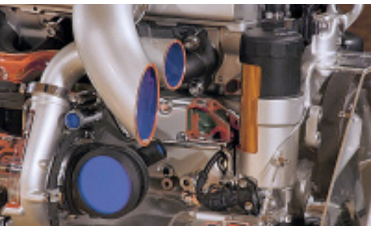
The oil and fuel filters are positioned upright in front of the engine for ease of service and maintenance.
