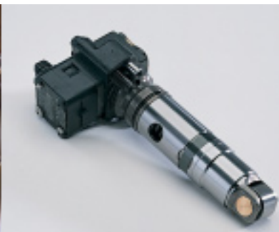
Electronically controlled injection features a unit pump injection system, with injection pressure up to 32,000 psi, for low emissions and excellent fuel economy.
