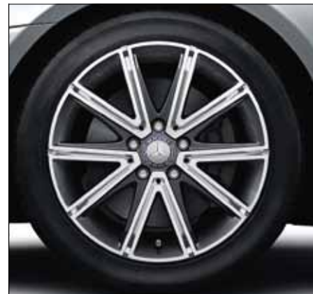
10-spoke light-alloy wheels, painted palladium silver, high-shine, with 225/45 R 17 front and 245/40 R 17 rear tyres (option, Code R93).
