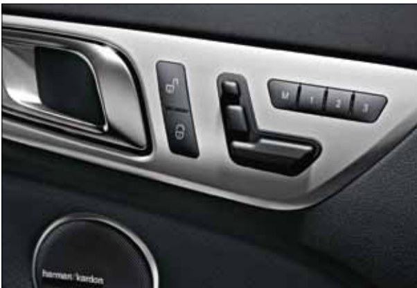
Electric seat adjustment with Memory function.
