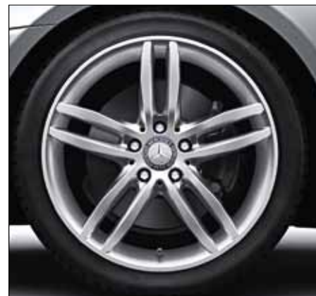
5-twin-spoke light-alloy wheels with 225/40 R 18 front and 255/35 R 18 rear tyres, exclusively for Sports package (option, Code R70).
