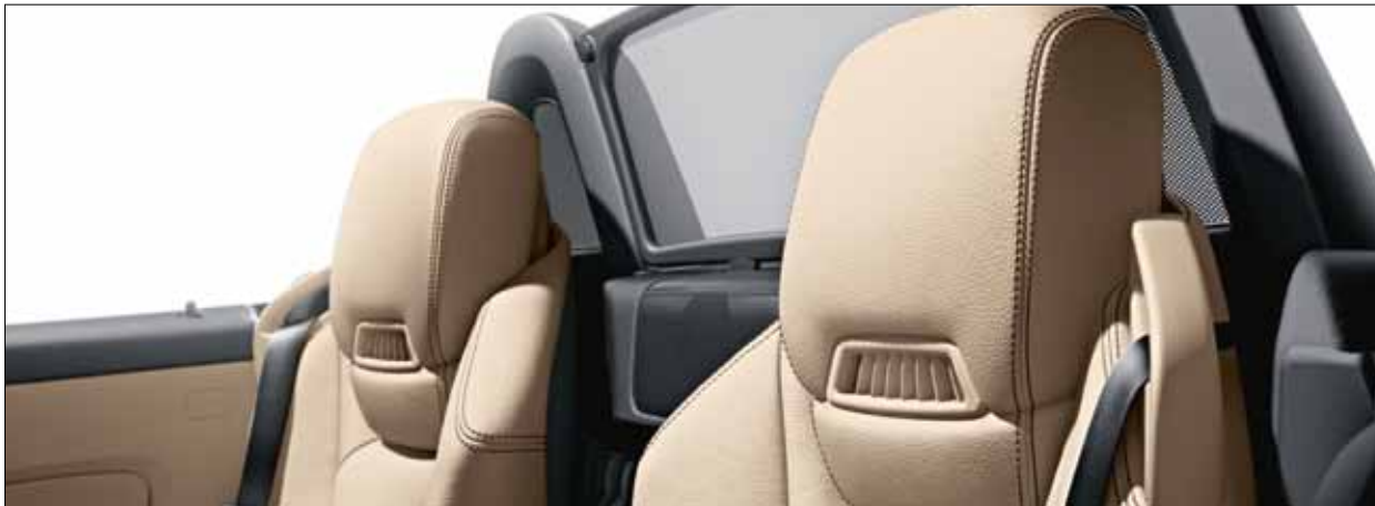
AIRSCARF delivers warm air to ensure perfect open-top motoring pleasure even in cool weather.
