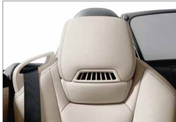
AIRSCARF neck-level heating.
