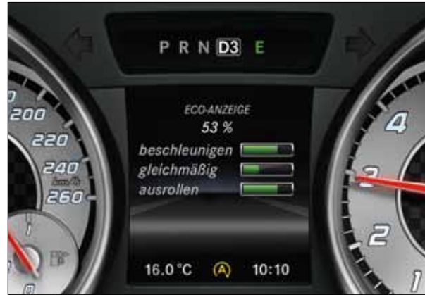
High-res display in instrument cluster (standard on SLK 350 and above). 1
