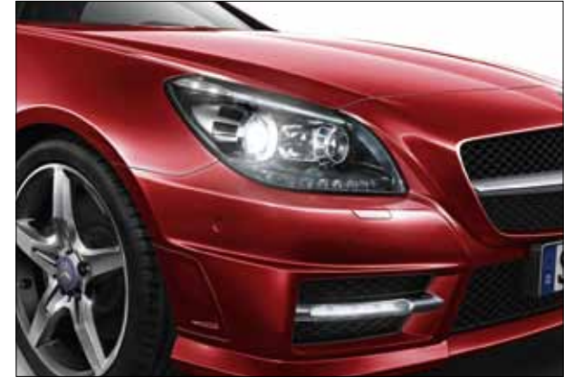
Intelligent Light System with LED daytime running lamps.
