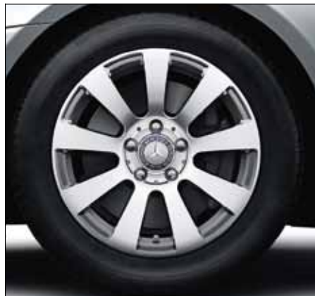
9-spoke light-alloy wheels with 205/55 R 16¹ tyres; 205/55 R 16 at front and 225/50 R 16 at rear (standard for SLK 250 CDI, Code R49).
