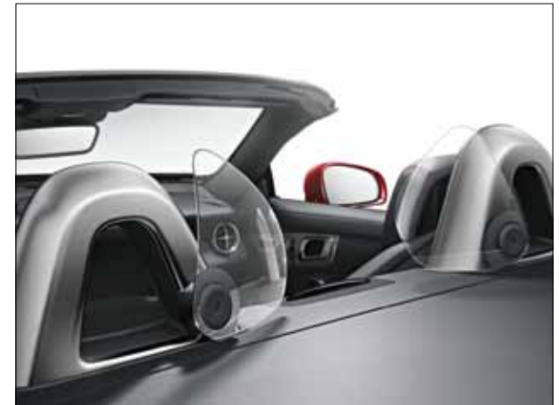
The draught-stop system AIRGUIDE minimises draughts in the interior of the open vehicle.
