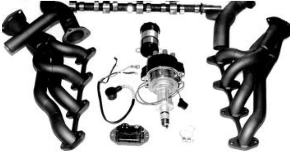
Headers, electronic ignition and camshaft.
