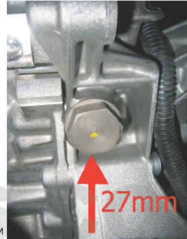
Chain Tensioner Torque: 80 NM
