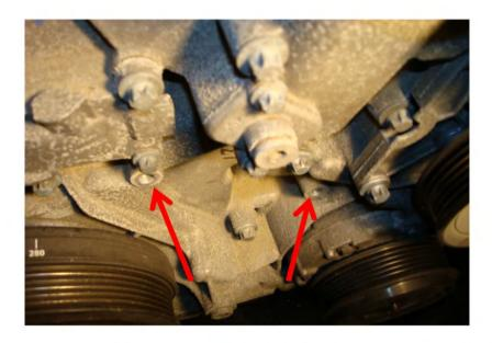
10) Install the new tensioner and torque the bolts to 25Nm (18 lbs ft) – and don't remove that pin yet!!
