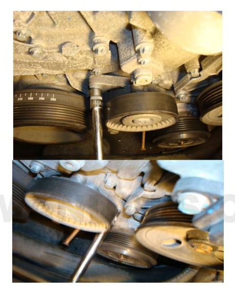
9) Once the old tensioner is removed, you may want to clean that area up and re-familiarize yourself where the mounting holes are. You may also want to clean up all the accessory pulleys (plain microfiber cloth or blow compressed air to remove any residual debris) as I found a good amount of sand/dirt in this area:
