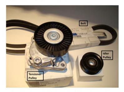
2) Do not remove the locking pin on the Tensioner Pulley – this pin will be removed after the new belt is installed:
