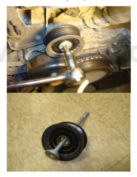
7) Clean the mounting area with a towel, and install the new idler pulley – there's no front or back but I like to have the part number visible. Torque to 20Nm (15 lbs ft).
