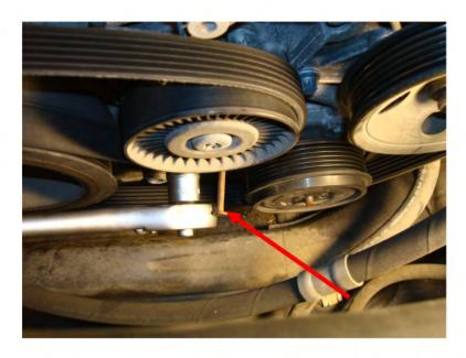
4) After locking the tensioner and removing the belt, it's a good time to check the water pump pulley for play. Hold it at either 9:00 or 3:00 and try to wobble it. If there's no play, there's no bearing problem with it (of course, the bolts holding the pulley to the water pump should be tight):
