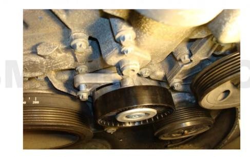
11) Install the new belt according to the belt path diagram – the tensioner pulley should be the last "loop" the belt passes around (or the water pump – you don't want to stretch the belt to get it over a pulley that has a lip on it) when you're installing the belt. Check the belt to make sure it is correctly seated on all the accessory pulleys.
