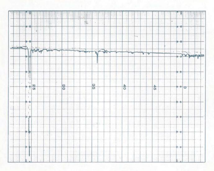
The signal strength recording shown on the page opposite was made in a New Jersey suburb, and shows flawless, undisturbed signal reception from a strong, local station.
