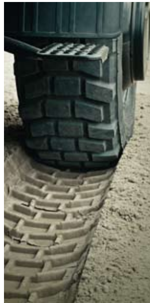
With tirecontrol you can adjust the tyre pressure to suit the terrain – simply with a switch
