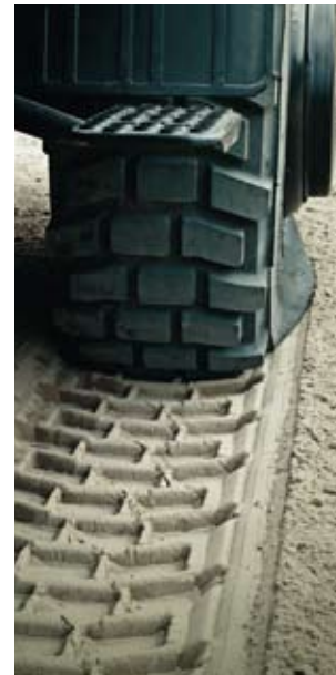
With tirecontrol you can adjust the tyre pressure to suit the terrain – simply with a switch
