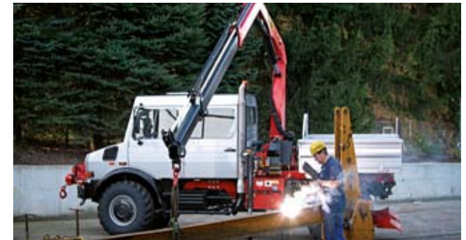
Commercially available hydraulic pumps, e.g. for a crane, can be used via a standardised connector on the auxiliary drive
