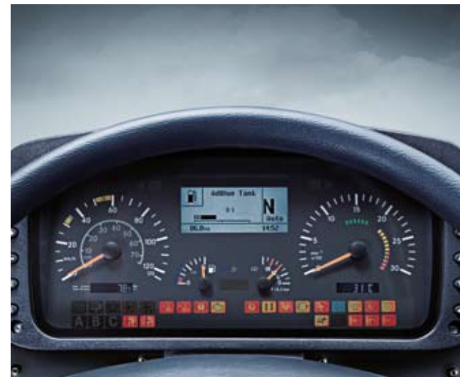
The instrument panel: clearly structured with an easy-to-operate driver information system (FIS), illuminated dials and 2 LCD multifunction displays
