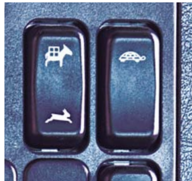
Rocker switch in the centre console for the basic, working and crawler gears.
