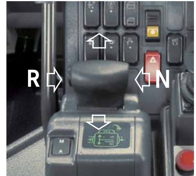
Switch between manual and automatic modes at the touch of a button.
