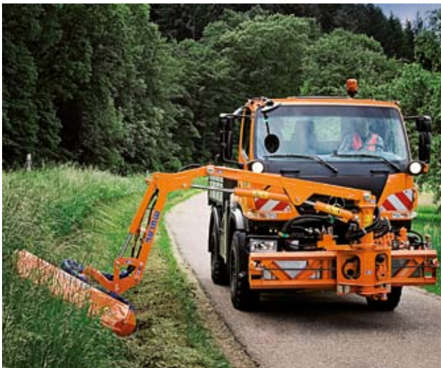
Sturdy front mounting plate for verge mowers, snowploughs or similar implements
