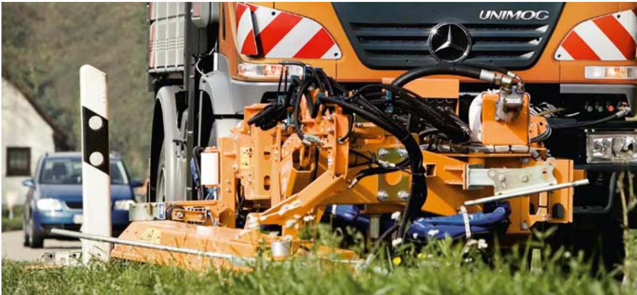
As a result of years of cooperation with leading implement and body manufacturers, the exceedingly powerful hydraulic system suits standard municipal implements perfectly
