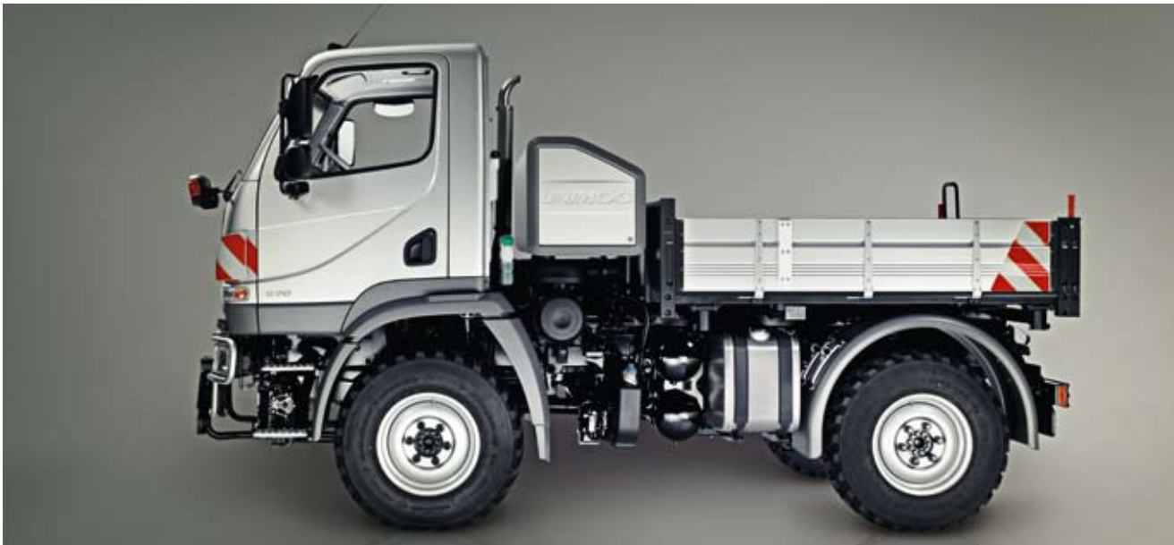
Short wheelbase, compact dimensions: the Unimog U20 is very manoeuvrable even in the most confined spaces, but still has a large frame for mounting implements
