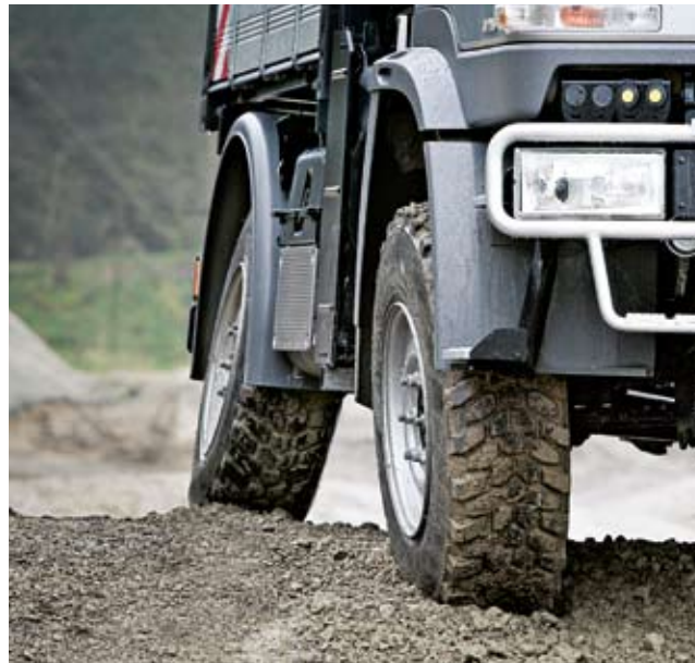
Outstanding off-road performance due to its axle articulation, permanent 4WD and manually engageable locking differentials in both axles
