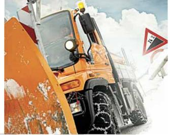
EQR (Electronic Quick Reverse). Completing the Unimog's winter service package is the preselectable electronic quick reverse (EQR) system. This synchromeshed forward/reverse shifting system allows frequent directional changes as required and makes clearing snow faster and easier.
