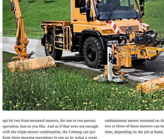
with the triple-mower combination, the Unimog can perform three mowing operations in one go by using a verge mower, a front boom embankment mower and a further
