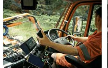
Taking the strain off the driver. The cab with its generous headroom and room to move, is made of non-corroding, noise and heat-insulating high-tech fibre composite material (FVW). It is very strong and rigid and with sprung and low-vibration mounting. As most of the functions are electrically controlled, the vibrations in the cab are reduced to a minimum. An optional air sprung driving seat is also available for yet more driving comfort.
