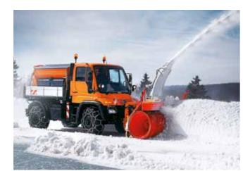
Front power take-off. Implements with high-power requirements up to 150 kW can be run from the powerful front engine-driven PTO.
