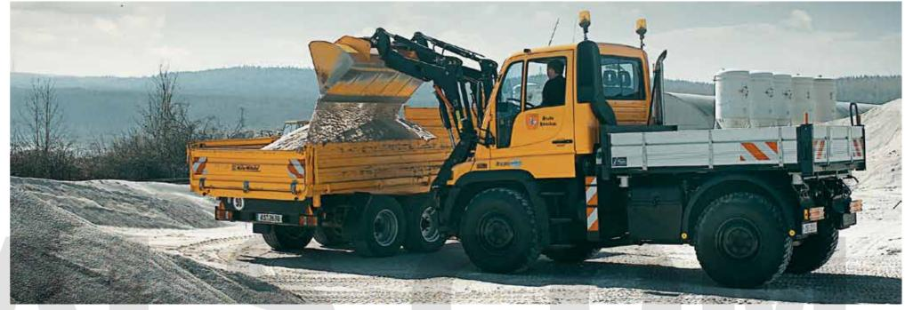
Fast and safe. The Unimog performs its transport jobs extremely reliably and especially quickly with maximum road speeds of 90 km/h. Not only does it get you to your destination quickly, it also gives you a very comfortable ride, even with a full load. And its safety features set standards, with four-channel ABS and automatic load-sensitive brake pressure control (ALB).
