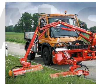
Endless possibilities. Whether for villages, towns or motorway maintenance departments, the Unimog can supply a suitable mowing combination for every requirement. For example, it offers one-person operation with a single mower fitted either at the front or at the rear. Or you can
