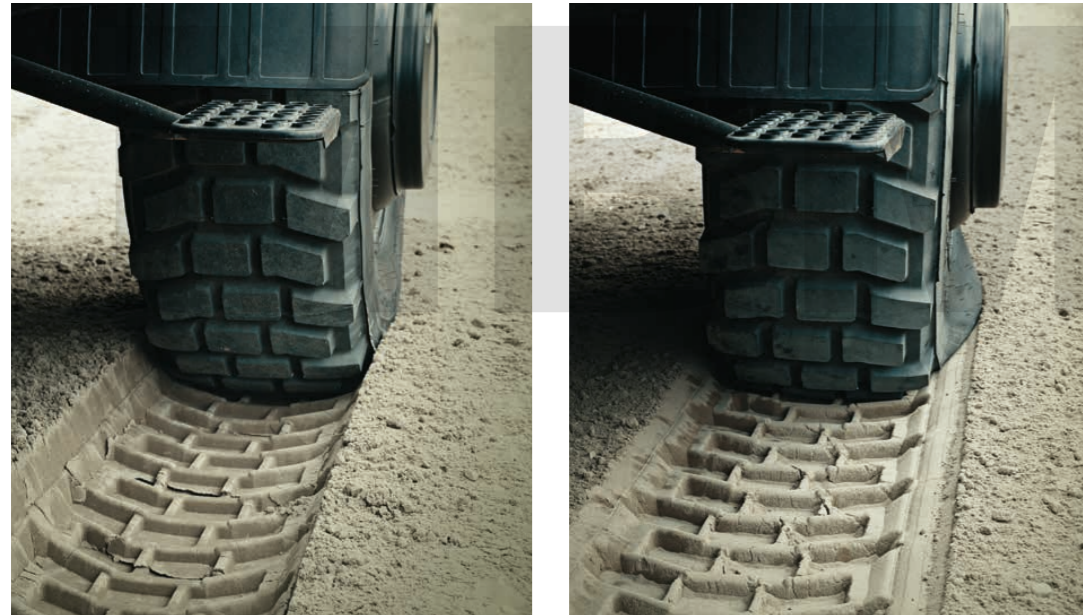
With tirecontrol/tirecontrol plus you can adjust the tire pressure to suit the terrain – simply with a switch
