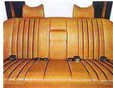
Adjustable rear seat with special headrests and three lap type seat belts.
