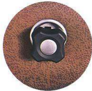
Seats hydraulically adjustable in longitudinal direction, height and backrest inclination by pressing a button
