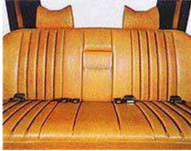
Three-point safety belts for the front seats and lap type for the rear seats. Special headrests.
