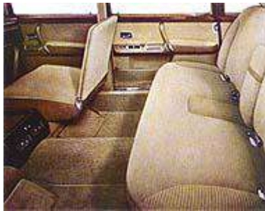
Six door model Fold-away seats in travelling direction, adjustable ducts for air-conditioning and controls for radio.
